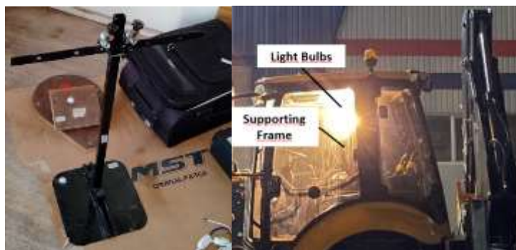
Figure 3. Lamp Source Apparatus (a) and Lamp Locations (b)
