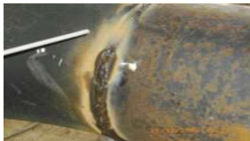
Fig.1: X70 pipeline steel after industrial arc welding
