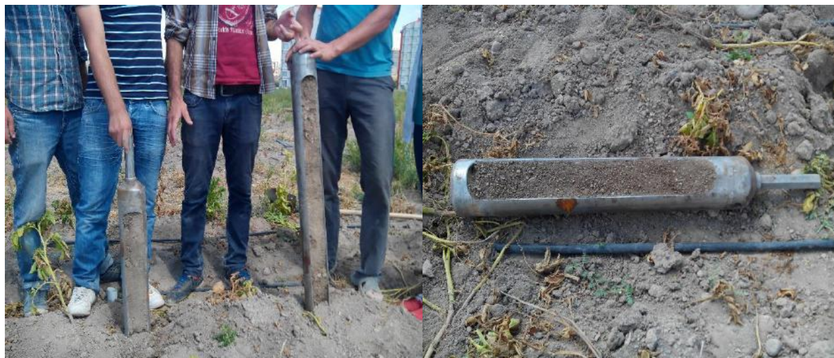
Figure 1. Destructive Soil Core Sampling from Freshly Harvested Area of Potato Field Experiment.
